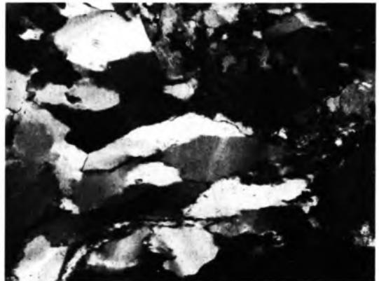
Fig. 3 : Development of quartz ribbons indicating intense ductile deformation
